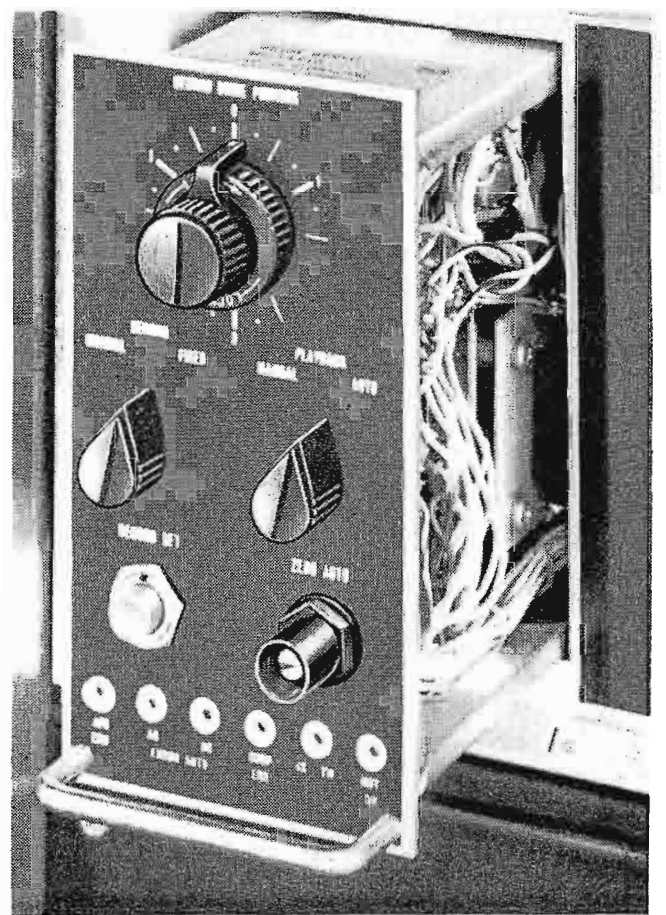
FIG. 15. Guide Servo accessory offers automatic as well as manual positioning of the vacuum guide.
