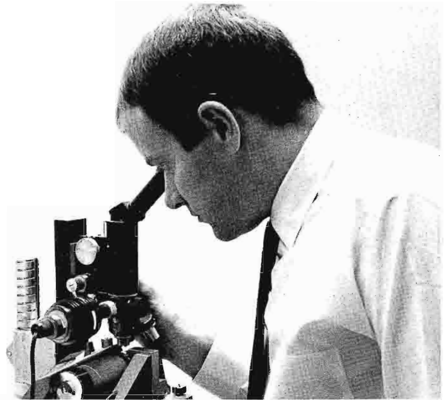
FIG. 6. Video head wear conditions can be evaluated by viewing the pole tips under a 150-power microscope with light attachment.
