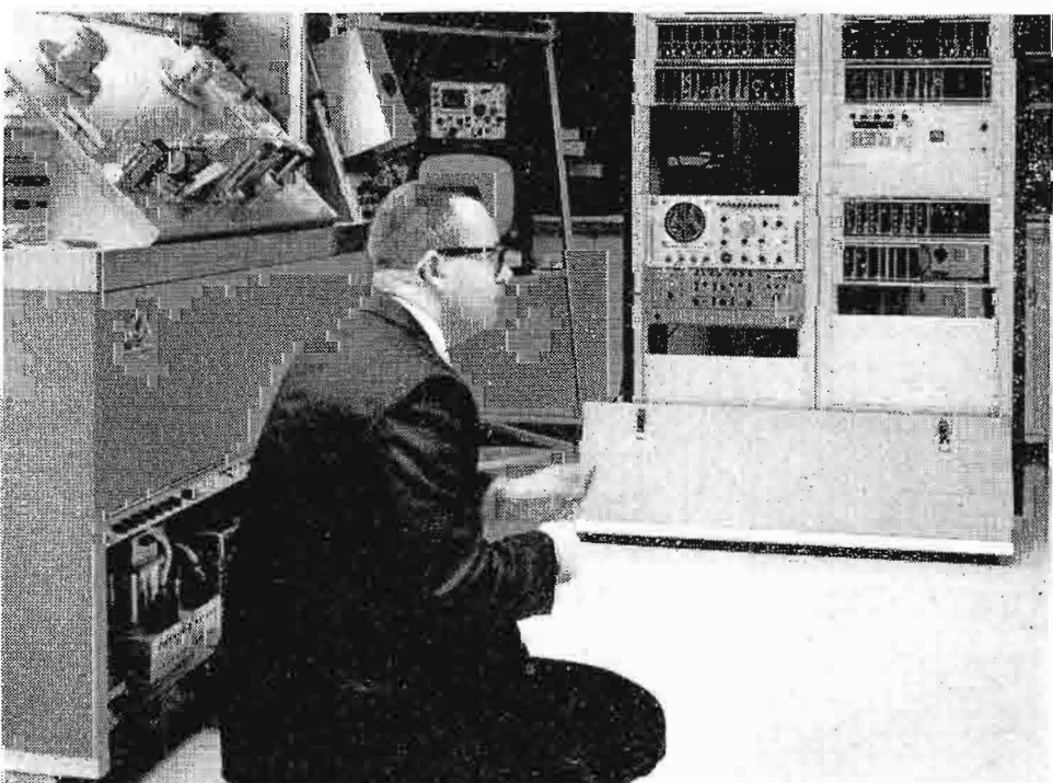
FIG. 20. Checking front access units of recorder.
